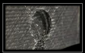
\* Image shows penetration of only the frontside of the sandwich panel because the inner core absorbed the impact
